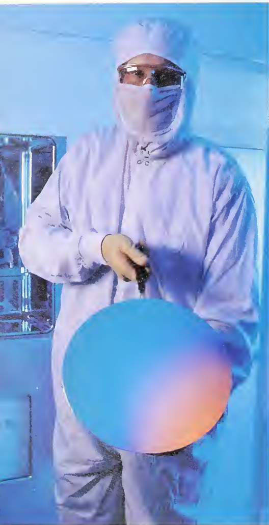
Worker holding the world's first 300 millimeter silicon wafer populated with electronic components using the wide beam ion implantation technology.
